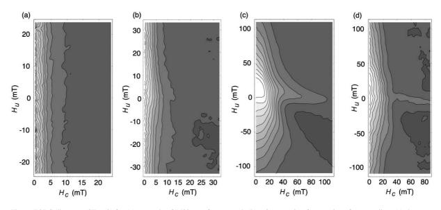
Fig. 6. FORC diagrams (SF = 3) for (a) a sample of M80 transformer steel; (b) a 2 mm grain of magnetite, after annealing; (c) the same 2 mm grain of magnetite before annealing; and (d) a  $125 \,\mu$ m magnetite grain (no annealing) from sample HM4 (see Hartstra, 1982).
